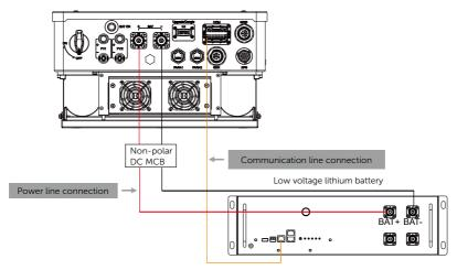
Figure 8-53 Lithium battery connection diagrm
