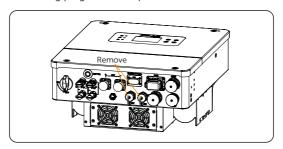
Figure 8-45 Removing the plugs
