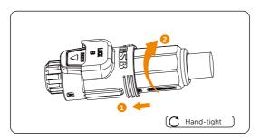
Figure 8-39 Tighten the body
