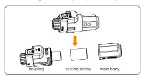
Figure 8-36 Disassemble the battery connector
