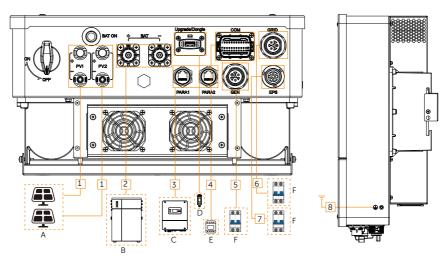
Figure 8-2 Cable connections of inverter
