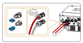
Figure 8-32 Connecting the PV cable
