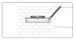
Figure 7-5 Marking the holes
