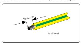
Figure 8-3 Striping the PE cable
