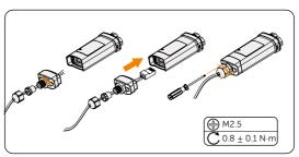
Figure 8-63 Assembling the dongle
