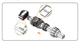
Figure 8-51 Insert the terminal into the body
