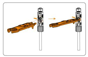
Figure 13-3 Disassembling the PV cables
