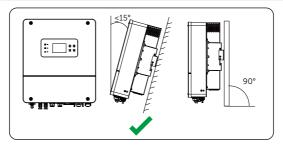
Figure 7-1 Correct installation
