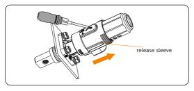
Figure 13-4 Open the latch and move the release sleeve
