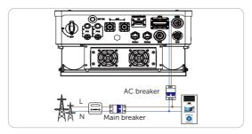
Figure 9-1 Turning on AC breaker
