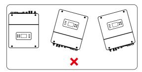
Figure 7-2 Incorrect installation
