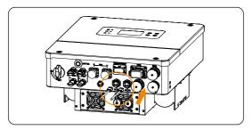
Figure 8-46 Insert the parallel wire
