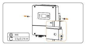
Figure 7-10 Securing the inverter
