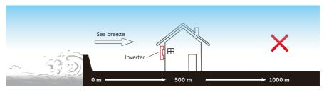
Figure 5-2 Incorrect installation position
