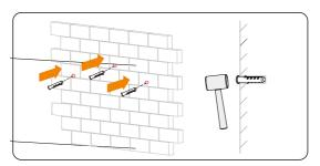
Figure 7-7 Insert the expansion tubes
