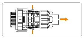
Figure 13-6 Releasing the communication cable
