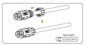
Figure 8-13 Tighten the nut
