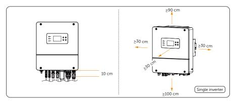
Figure 5-4 Clearance requirement for single inverters
