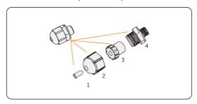
Figure 8-62 Disassembling the waterproof connector
