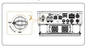
Figure 9-2 Turning on DC switch
