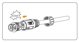
Figure 8-12 Insert the main body
