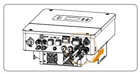
Figure 8-24 Plug the connector into the EPS, Grid and GEN terminal
