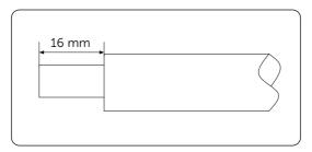
Figure 8-35 Stripping the battery cable
