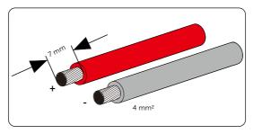
Figure 8-26 Stripping the PV cable
