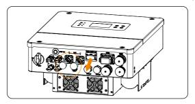
Figure 8-40 Remove the cap from the BAT terminal
