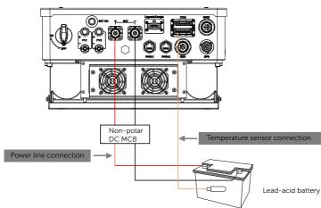
Battery temperature sensor connection diagram
