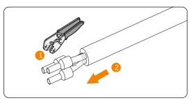
Figure 8-9 Sleeve the terminal onto the cable
