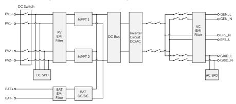
Figure 2-5 Circuit Diagram for X1-HYB-LV-EU series inverter
