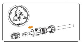
Figure 8-10 Set the parts on the cable
