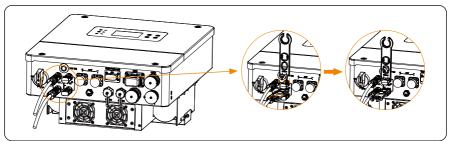
Figure 8-33 Disassembling the PV dustproof buckles
