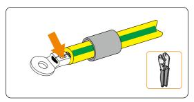
Figure 8-5 Crimping the cable
