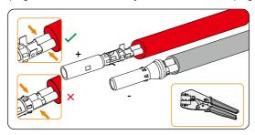
Figure 8-28 Crimping the terminal
