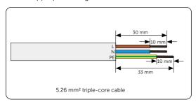
Figure 8-14 Stripping the Grid and GEN cable
