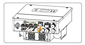
Figure 8-41 Plug the BAT connector into the BAT terminal
