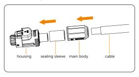
Figure 8-37 Insert the cable
