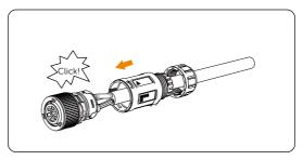
Figure 8-18 Insert the main body
