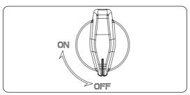
Figure 13-1 Turning off the DC switch
