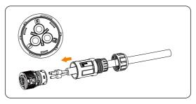
Figure 8-16 Set the parts on the cable
