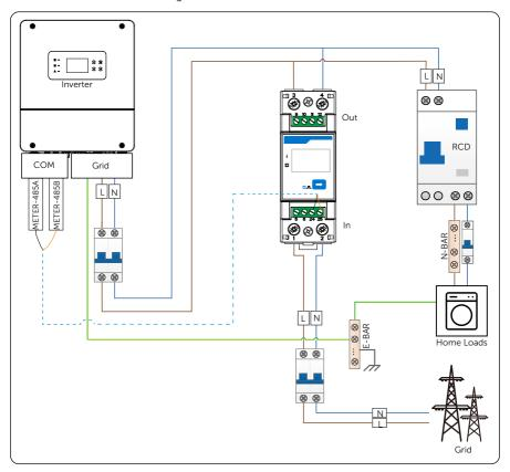
Figure 8-56 Meter connection diagram
