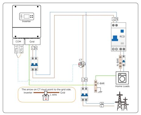
Figure 8-57 CT connection diagram
