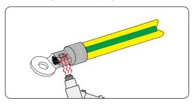
Figure 8-6 Shrinking the tubing
