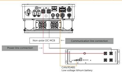
Figure 8-34 Battery connection diagram
