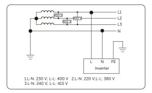
Figure 2-2 Supported power grid-TT
