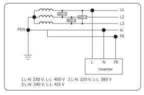
Figure 2-4 Supported power grid-TN-C-S
