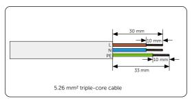
Figure 8-8 Stripping the EPS cable
