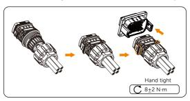
Figure 8-52 Connect to the COM port
