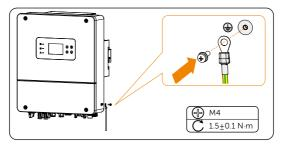
Figure 8-7 Securing the PE cable
