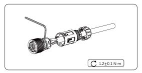
Figure 8-17 Crimping the wire
