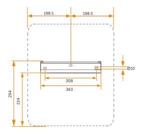
Figure 7-4 Dimensions 2 (Unit: mm)
