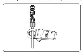
Figure 13-2 Measuring the current
