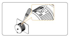
Figure 8-20 Flip the lock for EPS
