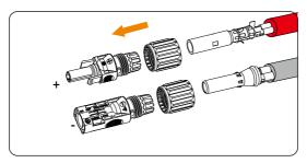
Figure 8-29 Threading the PV cable
