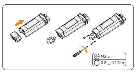
Figure 8-60 Assembling the dongle
