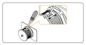
Figure 8-21 Flip the lock for Grid and GEN
