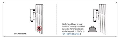
Figure 5-3 Installation carrier requirement
