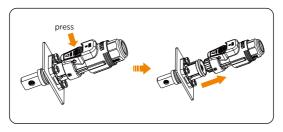
Figure 13-5 Pull out the plug
