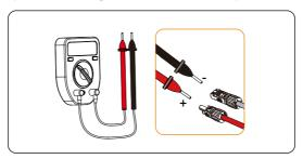
Figure 8-31 Measuring the voltage of PV connectors
