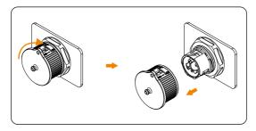
Figure 8-23 Remove the dust cover for Grid and GEN
