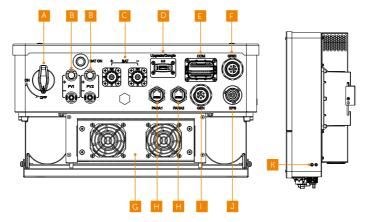
Figure 8-1 Terminals of Inverter
