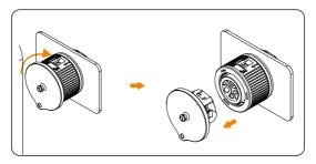
Figure 8-22 Remove the dust cover for EPS
