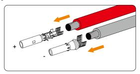
Figure 8-27 Inserting the PV pin contact
