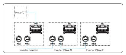
Figure 15-11 Communication wiring
