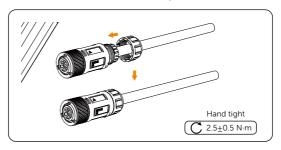
Figure 8-19 Tighten the nut
