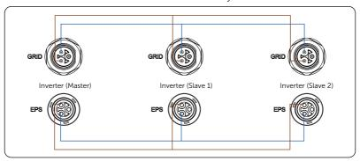
Figure 15-10 Power cable wiring
