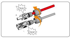
Figure 8-30 Securing the swivel nut
