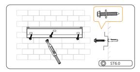
Figure 7-8 Securing the bracket
