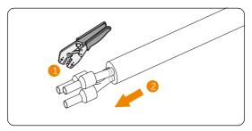
Figure 8-15 Sleeve the terminal onto the cable
