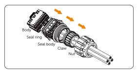
Figure 8-50 Set parts on the cable
