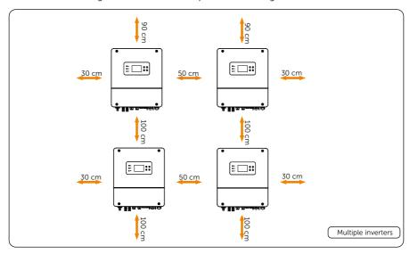
Figure 5-5 Clearance requirement for multiple inverter
