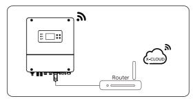
Figure 8-59 LAN mode connection diagram
