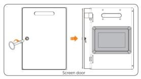
Figure 10-2 Unlocking screen door
