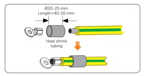
Figure 7-4 Attaching tubing and ring terminal
