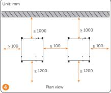
Figure 4-35 Clearance requirements for multiple cabinets
