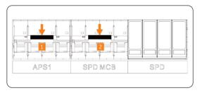
Figure 11-4 Flipping down breakers on distribution box (2)
