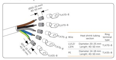
Figure 7-15 Attaching tubing and ting terminals
