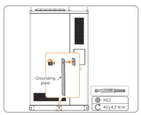
Figure 7-2 Securing grounding plate
