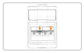
Figure 11-8 Flipping down high-voltage box breakers
