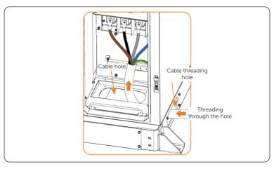
Figure 7-17 Threading the cable
