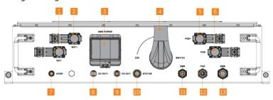
Figure 2-12 Appearance of high-voltage box
