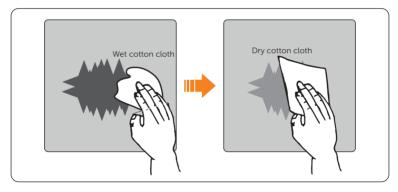
Figure 14-5 Cleaning the scratched area
