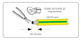
Figure 7-3 Striping cable jacket
