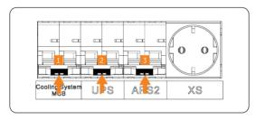
Figure 8-4 Flipping up breakers on distribution box (2)
