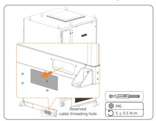
**Step 7:** Thread one end of the network cable through the reserved cable hole and cable threading hole in sequence.
