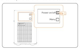
Figure 11-9 Shutting down the UPS
