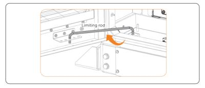
Figure 7-9 Placing the limiting rod
