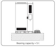
Figure 4-31 Foundation requirement
