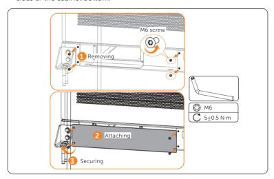
Figure 6-45 Fixing cover plate
