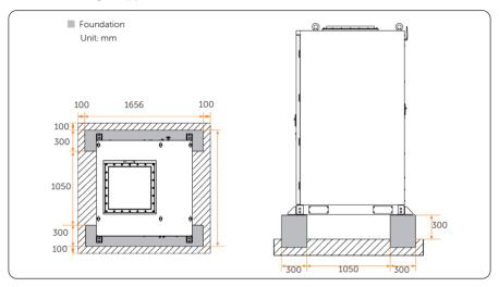
Figure 4-32 Foundation requirements for angle supports installed at front and rear sides
