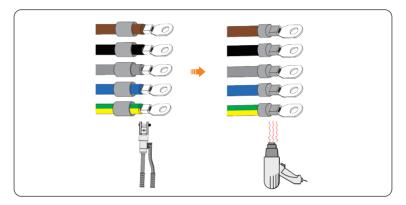
Figure 7-16 Crimping and heating the wires
