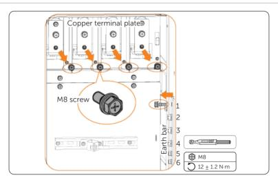
Figure 7-11 Unscrewing screws
