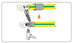
Figure 7-5 Crimping and heating
