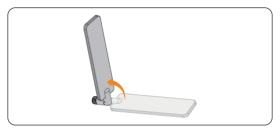
Figure 6-48 Folding up antenna stick
