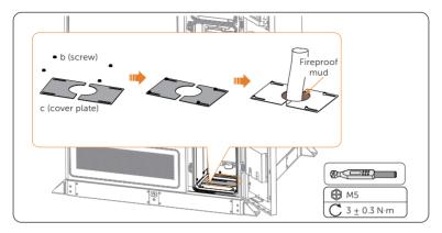
Figure 7-21 Sealing the cable hole
