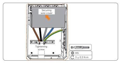
Figure 7-20 Securing cable clamp and wire cover
