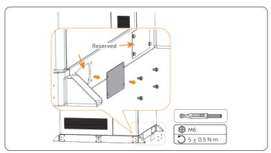
Figure 7-7 Removing the cover for cable threading hole
