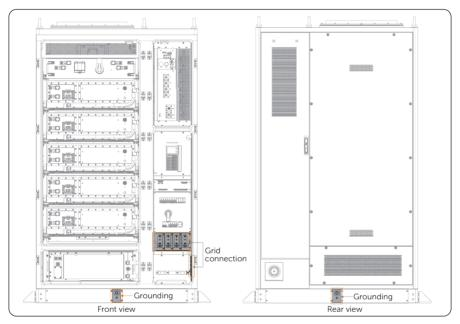
Figure 7-1 Position of the wired parts
