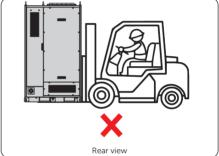
Figure 6-40 Improper way of handling
