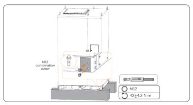
Figure 6-41 Removing M12 screws
