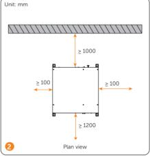
Figure 4-34 Clearance requirements for a single cabinet
