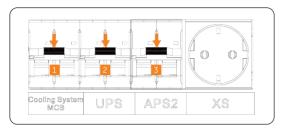
Figure 11-3 Shutting down breakers on distribution box (1)
