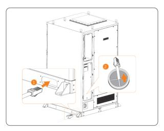
Figure 7-27 Threading through the network cable
