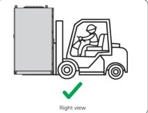
Figure 6-39 Proper way of handling
