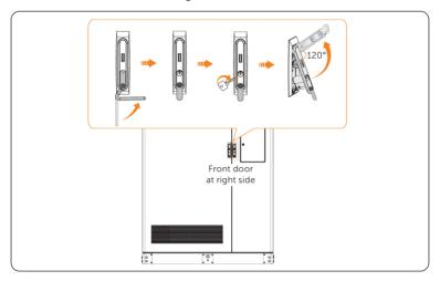
Figure 7-8 Unlocking the front door
