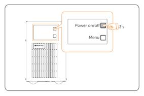
Figure 8-5 Holding and pressing button
