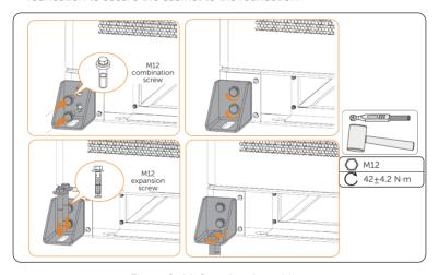
Figure 6-44 Securing the cabinet
