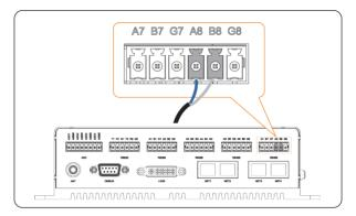
Figure 7-31 Connecting communication cable to EMS1000
