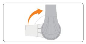
Figure 11-7 Switching off the high-voltage box
