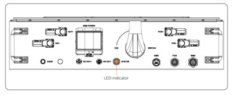
Figure 9-10 High-voltage box LED indicator
