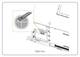
Figure 7-26 Cutting open the seal of cable hole
