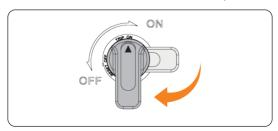
Figure 8-2 Switching on the distribution box
