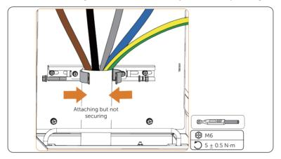
Figure 7-18 Reattaching the cable clamp
