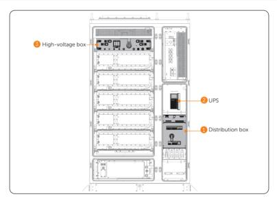
Figure 8-1 Position of modules for powering on system
