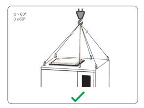
Figure 6-37 Proper way of hoisting
