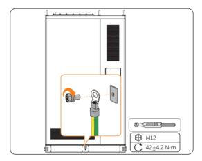
Figure 7-6 Securing PE cable
