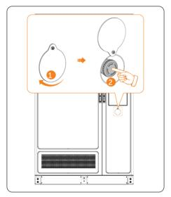
Figure 11-10 Pressing emergency stop button
