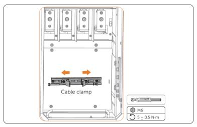
Figure 7-12 Removing cable clamp
