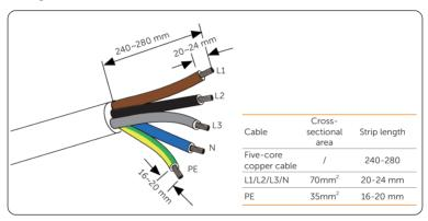
Figure 7-14 Striping wires
