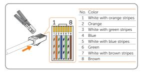
Figure 7-23 Crimping RJ45
