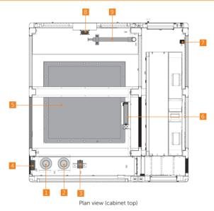
Figure 2-9 Parts on the cabinet top
