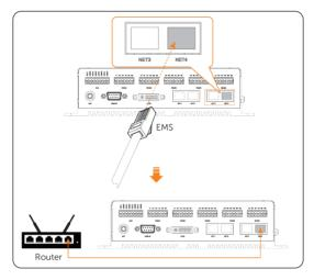
Figure 7-29 Connecting the network to EMS and switch
