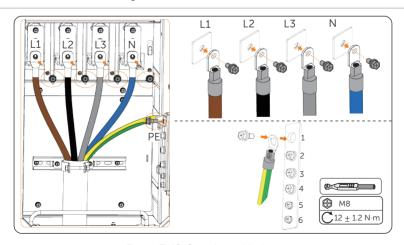
Figure 7-19 Securing grid wires
