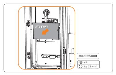
Figure 7-10 Removing cable cover
