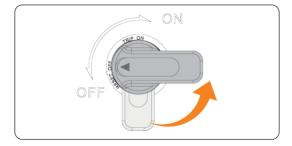
Figure 11-6 Switching off the distribution box
