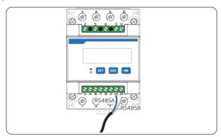
Figure 7-32 Connecting communication cable to meter
