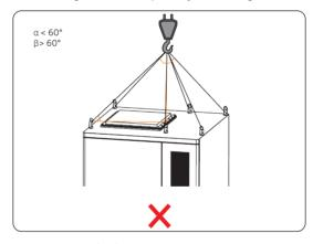
Figure 6-38 Improper way of hoisting
