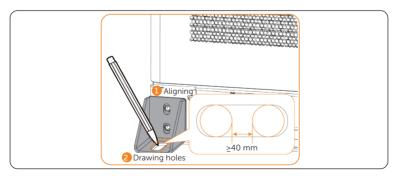
Figure 6-42 Aligning and drawing holes
