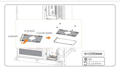
Figure 7-13 Removing fireproof mud panel
