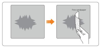
Figure 14-4 Sanding the scratched area
