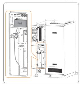
Figure 7-28 Running the Ethernet cable
