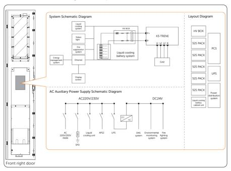
Figure 2-28 Position and content of the label
