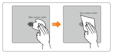
Figure 14-2 Cleaning the scratched area
