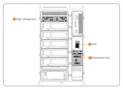
Figure 11-1 Position of modules for normally powering off system
