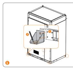
Align the holes in the cabinet, Draw circles on the ground.
